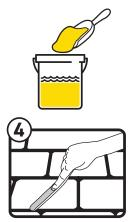
• Once joints are filled, remove excess product from the surface and then continue rinsing the entire area thoroughly while brushing.
