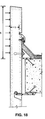
WIND LOADING OF PARAPET WALLS (See Fig. 18)
