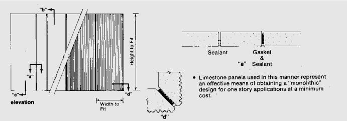
· Panels are normally anchored at top and bottom with no mechanical anchorage at the vertical joints-thereby creating a flexibility whereby the panels can easily be removed and reused if building is expanded.
