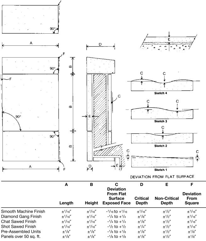
Tolerances C and F are measured within the length of a standard 4'-0" straightedge applied at any angle on the face of the stone.
