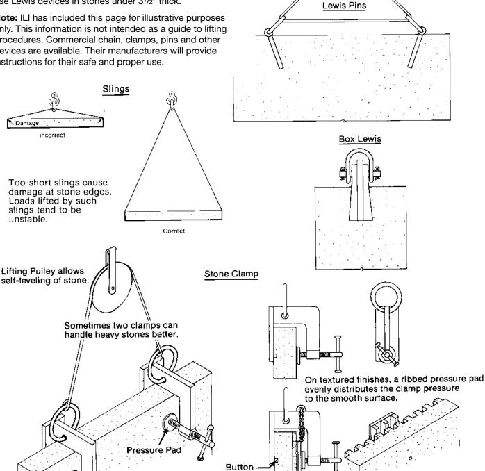
Chain retains ribbed pressure pad from falling when loosened.
