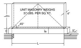
The Beam & Lintel Table is based on a rectangular loading pattern as shown. The actual loading by unit masonry when mortar sets approximates a triangle as shown by the dotted lines. Therefore, the table is conservative.
