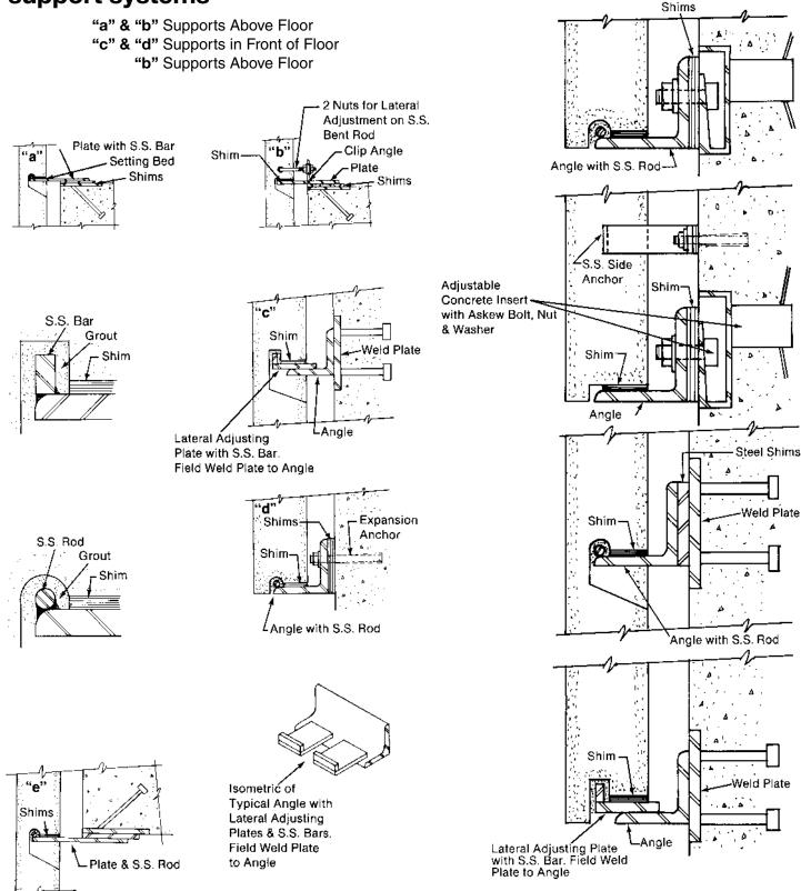
**Note:** The preferred location of gravity shelves is in the bottom bed or at least in the bottom 1/3 of the panel.
