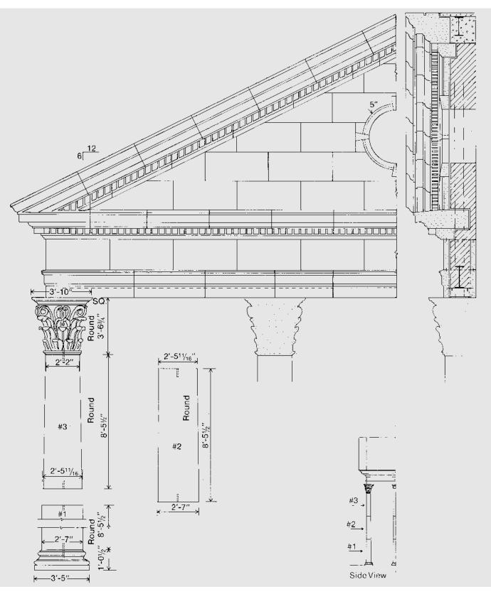
Column drum beds, and the beds of column bases and capitals, should be matched to their membering surfaces in the mill prior to shipment. The stone fabricator has the responsibility to produce column parts to the tolerance allowed for other "critical depth" situations.
