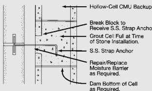
S.S. Strap Anchor Inserted into Broken CMU and Secured by Grouting Cell Full.
