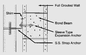
S.S. Strap Anchor Expansion Anchored to Solid CMU.
