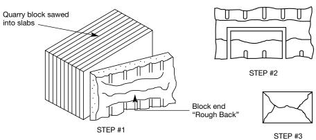
STEP #1—A sawed-6-sides stone slab is drilled and split to obtain two pieces of rock face.
