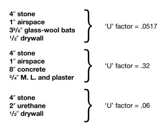
as U = 1/R total. In these examples, a constant figure for 4" stone is used to show the comparative values of three types of wall construction:
