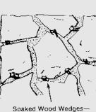
to be Removed After Mortar Sets Up
