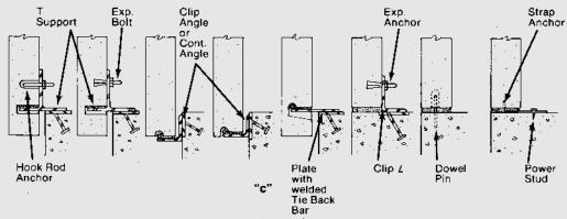
Note: In using expansion bolts as tie backs, refer to manufacturer's instructions regarding distance to any edge, and distance from center-line to center-line.
