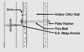
S.S. Strap Anchor Expansion Anchored to Hollow CMU. Note: Use This Type of Anchor for Heavy Loads.
