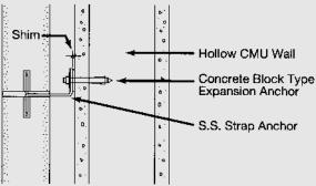
S.S. Strap Anchor Expansion Anchored to Hollow CMU. Note: Use This Type of Anchor at Light Loads Only.
