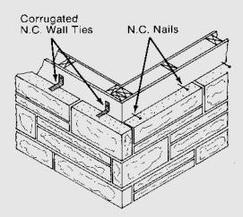
Stone Veneer Anchored to Wood Frame Backing
